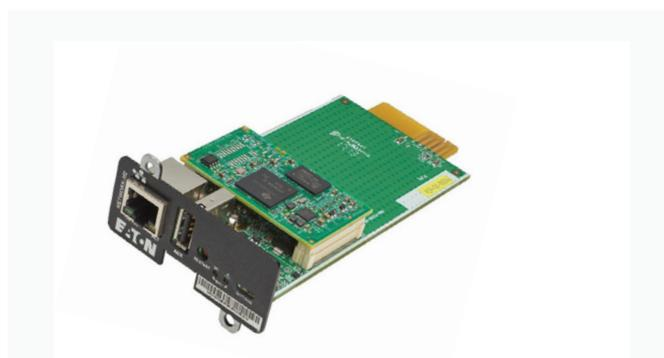
The first UPS connectivity device to meet both UL and IEC cybersecurity standards.
