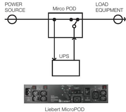
When your computer system can not be without power, even for scheduled UPS maintenance, the Liebert MicroPOD Maintenance Bypass and Output Distribution Unit ensures continuous uptime. It allows you to manually transfer connected equipment to utility power via a maintenance bypass switch, permitting scheduled service or UPS replacement without the need to shut down connected equipment.
