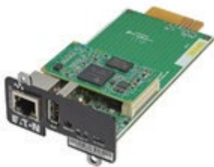
Network-M2 Giga bit network card.
