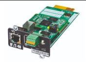
The Eaton Industrial Gateway Card (INDGW-M2) combines the features of an SNMP agent, HTTP/web server and a Modbus card to facilitate remote monitoring of your UPS system through any Building Management System. Enjoy the freedom to customize and schedule actions, like shutdown protocols and load shedding, and receive immediate notifications during power events, without having to be onsite.
